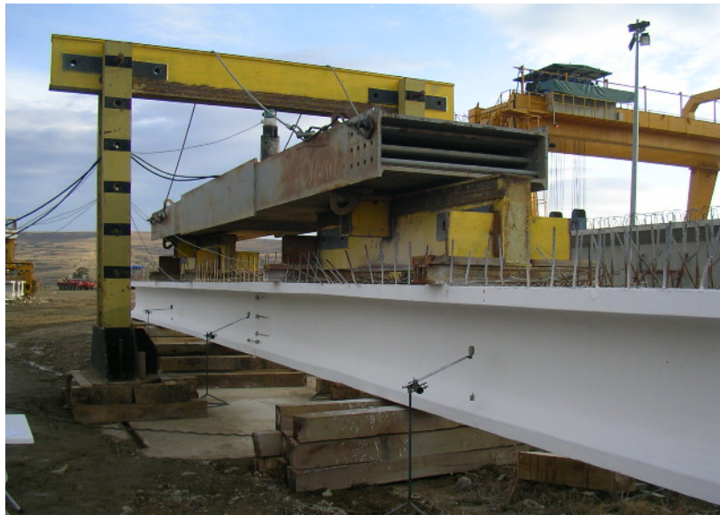
Figure 4. T- 24m beam in the test stand in Săvădisla Camp
