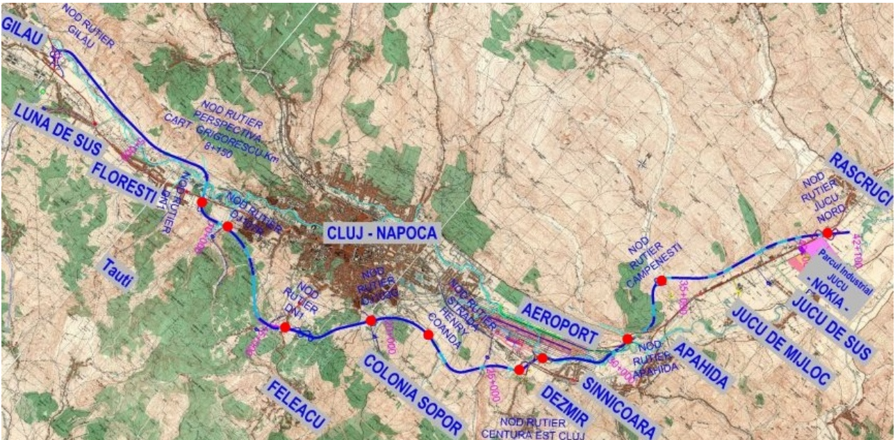
Figure 5. Alignment of the Cluj-Napoca Urban Motorway as it resulted from the feasibility study
