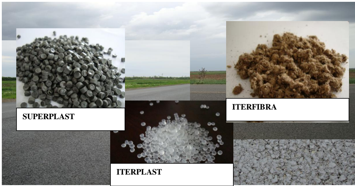
Figure 4. Products used at asphalt mixtures manufacturing
