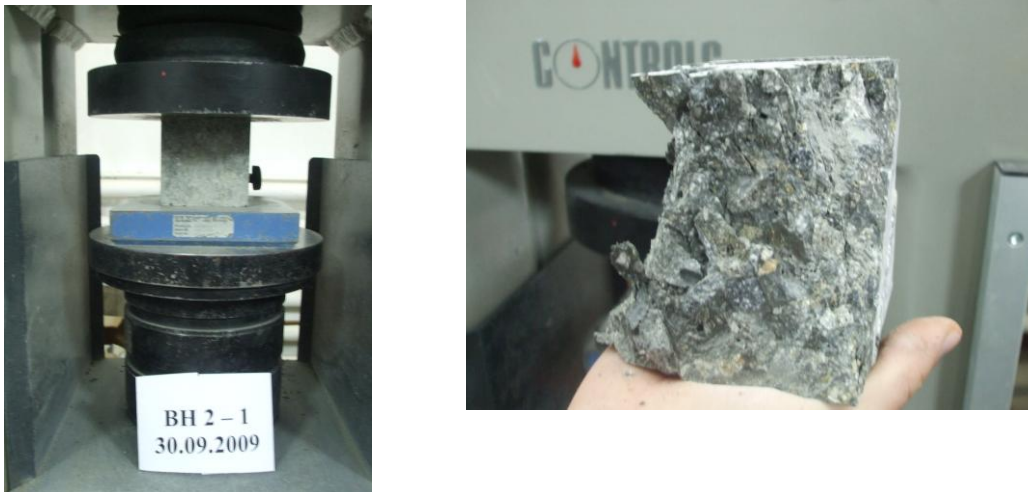
Fig. 1. Compressive strength test on cubes, in the Advantest press.
