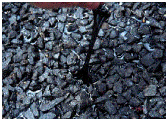
Figure 2. Mixture with modified bitumen
