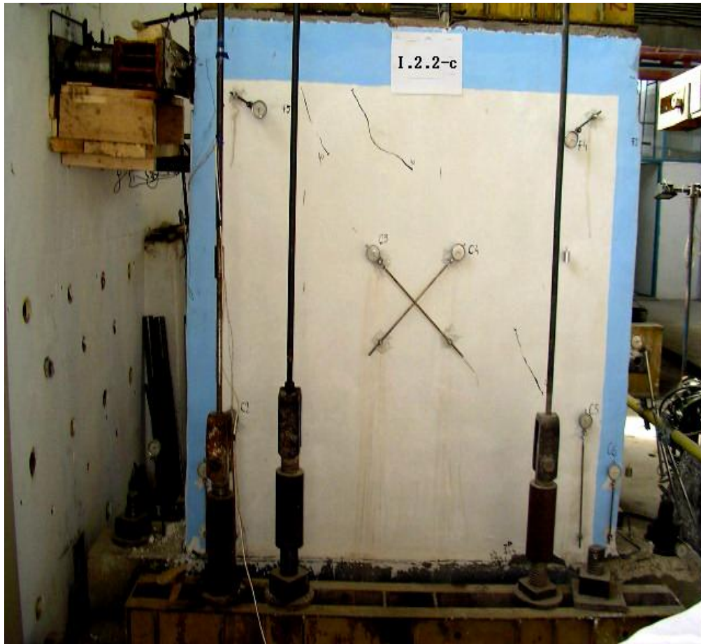
Fig. 7. Equipping of the trial stall for the consolidated masonry element
