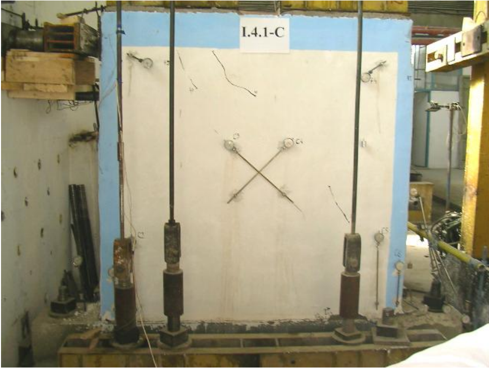
Fig. 3. Equipping of the trial stall for the consolidated masonry element
