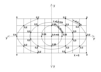
Figure 9. Isokinetic curves for  $\overline{x} = 6$ .
