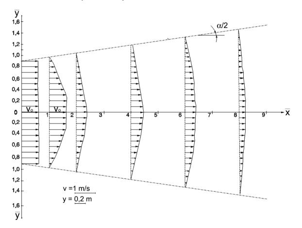
Figure 3. Air velocity hodographs measured in horizontal plane.
