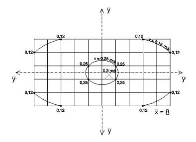
Figure 10. Isokinetic curves for  $\overline{x} = 8$ .
