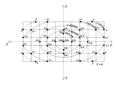
Figure 8. Isokinetic curves for  $\overline{x} = 4$ .
