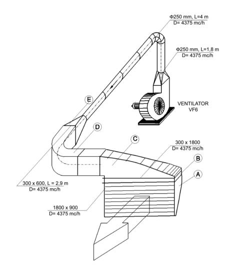
Figure 2. Stand for studying the air velocity field of the double-equal strength inlet device (double-exponential profile)– Isometric drawing.
