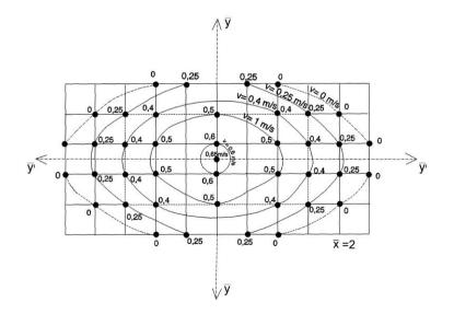
Figure 7. Isokinetic curves for  $\overline{x} = 2$ .
