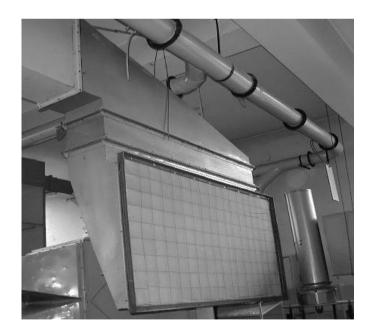
Figure 1. Stand for studying the air velocity field of the double-equal strength inlet device (double-exponential profile) for spatial air-distribution.
