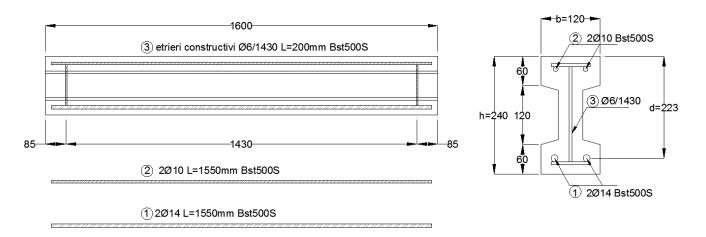
Fig. 2 - Reinforcement layout and geometric characteristics for ultra-high performance fiber reinforced concrete beam.
