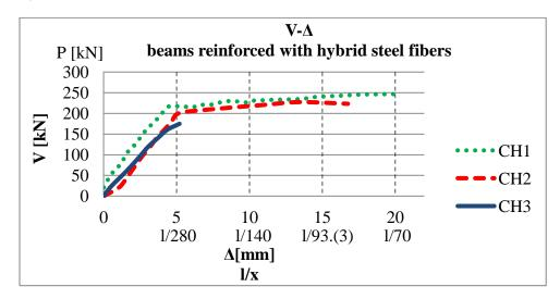
*Fig.* 5 – *Force-deformation diagram for beams reinforced with hybrid steel fibers.*
