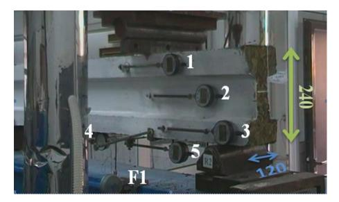
*Fig.* 3 – *testing equipment:* 1,2,3  $\rightarrow$  *digital strain gauges;* 4,5  $\rightarrow$  *digital strain gauges measuring reinforcement deformation;* F1  $\rightarrow$  *deformeter for measuring*  $\Delta$  *deformations.*
