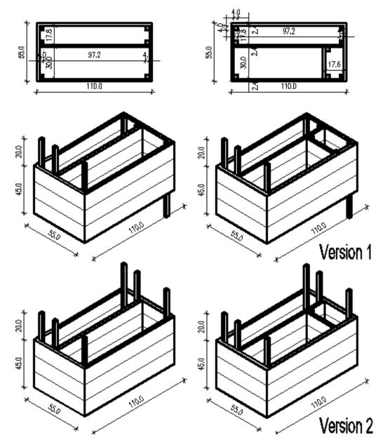
Figure 3. Wooden box module, example for field and corner
