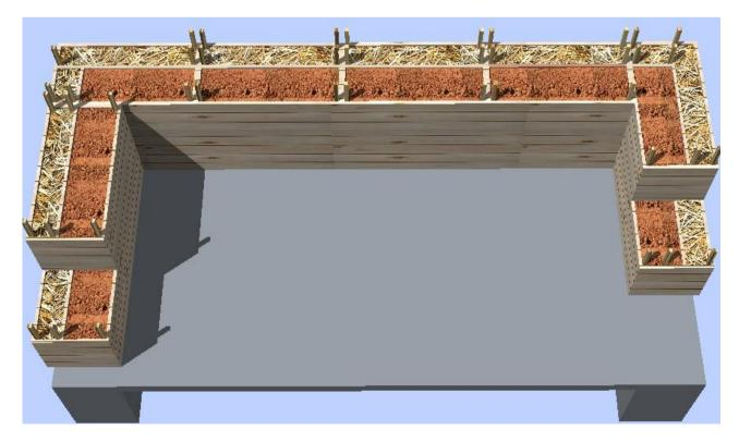
Figure 4. Example of wall built using the box-module
