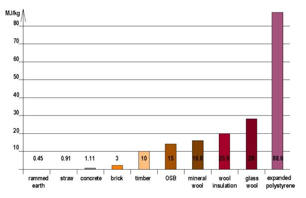
Figure 1. Embodied energy of common building materials
