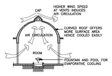
Figure 7. Induced ventilation through curved roof and air vents
