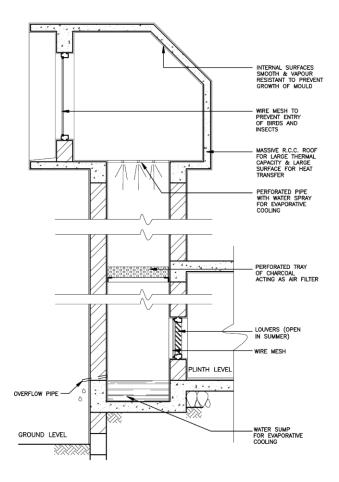
Figure 8. Section showing detail of a wind tower.
