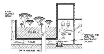
Figure 10. Working principle of earth air tunnel.
