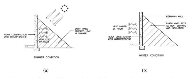
Figure 11. Working principle of earth berming during summer (a) and winter (b) conditions.
