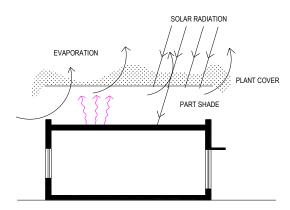
Figure 3. Roof shading by plant cover.
