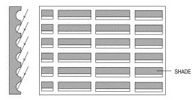
Figure 6. Shading due to surface texture
