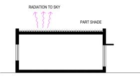
Figure 4. Roof shading by earthen pots.
