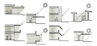
Figure 1. Different types of shading devices.
