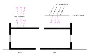
Figure 2. Roof shading by solid cover.
