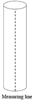
Figure 1 – Measuring line on cylindrical specimens, having a diameter of 150 mm and height of 300 mm
