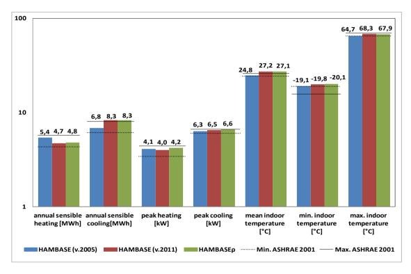
Figure 6. Comparison between different versions of Hambase vs. ASHRAE 140/2001 (logarithmic scale)
