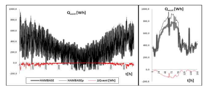
Figure 4. HAMBASE vs. HAMBASE p - heat loss through air ventilation (case 600) for one year (left) / first week (right)
