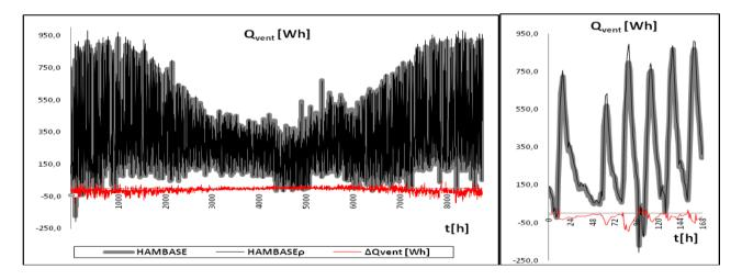
Figure 3. HAMBASE vs. HAMBASEp - heat loss through ventilation air (case 600ff) for one year (left) / first week (right)
