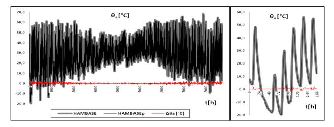
Figure 2. HAMBASE vs. HAMBASEp - indoor air temperature (case 600ff) for one year (left) / first week (right)
