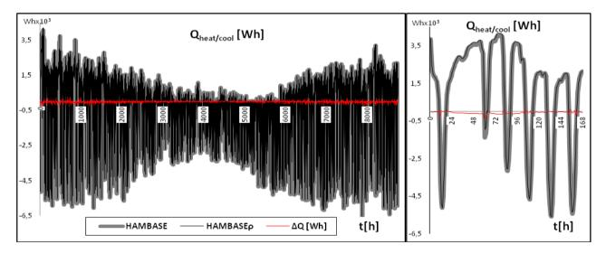
Figure 5. HAMBASE vs. HAMBASEp - hourly loads heating/cooling (case 600) for one year (left) / first week (right)
