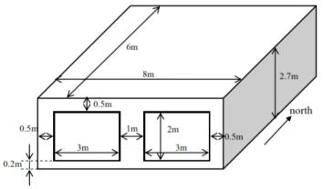
Figure 1. Reference building used in the ASHRAE Bestest 140/2001 [7]
