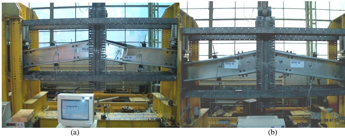
Figure 3. Failure of ridge specimens RIP-M (a) and RIS-FB-M (b)
