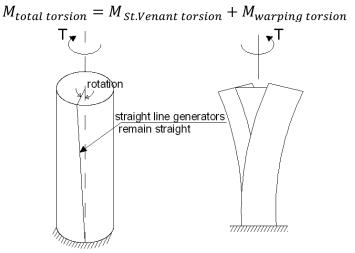
Figure 1. a) St Venant torsion b) warping torsion [2]
