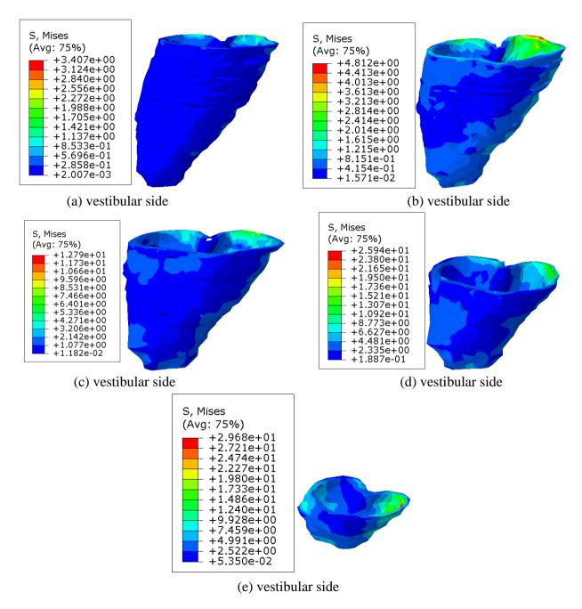
Fig. 2. presents the von Mises stresses distribution within the peridontal ligament having a resorption degree of (a) 50%, (b) 60%, (c) 70%, (d) 80%, (e) 90%.
