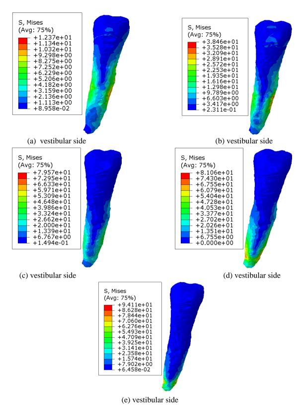
Fig. 1. presents the von Mises stresses distribution within the tooth having a surrounding support tissues resorption degree of (a) 50%, (b) 60%, (c) 70%, (d) 80%, (e) 90%.
