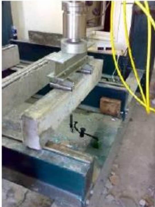
Fig. 8. Testing frame and loaded beam.
