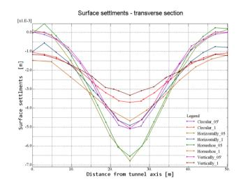
Figure 7. Surface settlements for analyses with k=1 and k=0.5.
