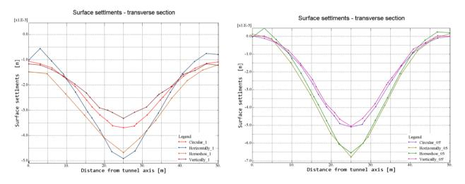
Figure 6. Surface settlements for analyses with k=1 (left) and k=0.5 (right)
