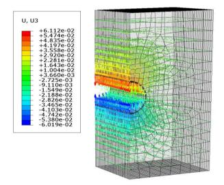
Figure 8. Displacement vector plot for u3, circular k=1.
