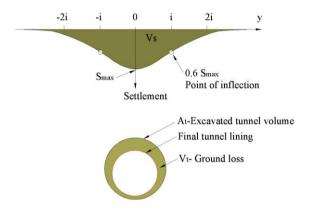
Figure 1. Transverse settlement – Gaussian curve. [3]
