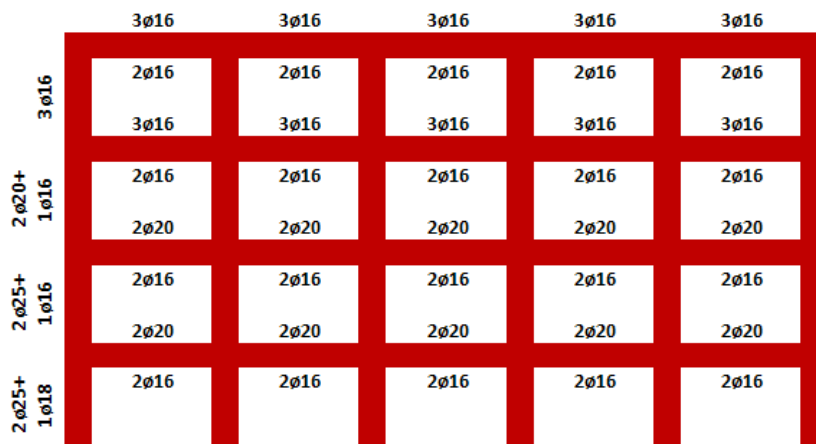
Fig.3. Reinforcement of the beams (total) and columns (side reinf.), existing 4 storied structure
