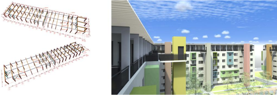
Figure 9. Structural frames of the “attic”.
