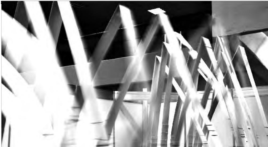
Figure 18. Responsive behavior of the physical system - detail with the flexible modulated elastic structure made out of balsa wood.
