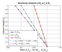
Fig. 5. Sensitivity analysis of  $E_c$  with  $W_c$  and  $f'_c$  according to column nonparametric height ( $K_w$ =0.95 &  $K_c$ =0.90)
