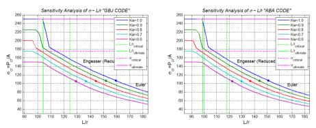
Fig. 16.  $P_{u}/P_0=1$ ,  $\rho=\%2$ , e=0,  $I_m=0.65I_g$ , left GBJ code, right ABA code.  $K_w=0.6$  to 1
