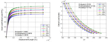
Fig. 11. Critical Load change with  $\delta/L$  and L/r ratios according to different codes
