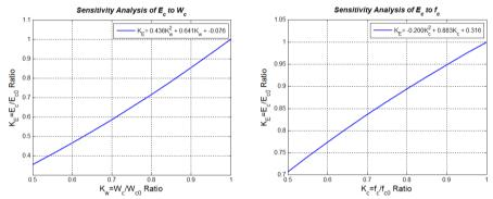
Fig. 3. Sensitivity analysis of Ec with Wc and f'c according to different  $K_w$  and  $K_c$  ratios
