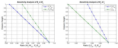
Fig. 4. Sensitivity analysis of  $E_c$  with  $W_c$  or  $f'_c$  according to column nonparametric height left:  $K_w$ =0.95, right:  $K_c$ =0.90)
