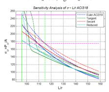
Fig. 13. Buckling stress versus slenderness for various types of modulus theories and ACI-318 code. I=1.0 $I_g$ , (-) $K_w=0.9$ , (-.)  $K_w=1.0$
