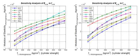
Fig. 7. Relationship curves of elasticity modulus and various concrete strengths for different design codes, left:  $K_c=0.9$ , right:  $K_c=0.6 [K_c=f'_c/f'_{c0}]$
