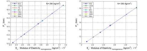
Fig. 10. Elastic modulus change with critical load according to different codes, (left  $K_w$ =1, right  $K_w$ =0.8)
