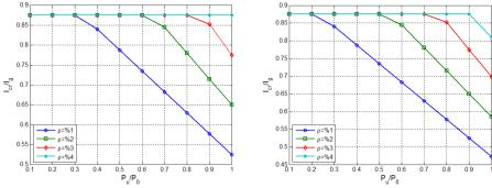
Fig. 8. Cracked moments of inertia of compression and flexural members according to different reinforcement ratios, left  $e=0, M_u=0, \text{ right } e=\%5, M_u=0.05*h*P_u$
