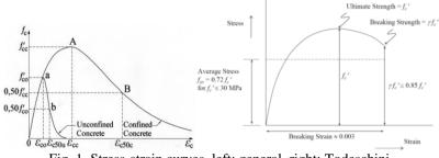
Fig. 1. Stress-strain curves, left: general, right: Todeschini
