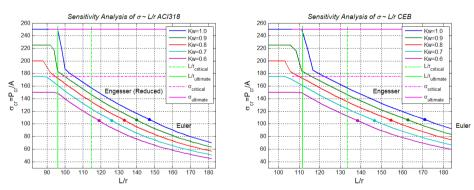
Fig. 14.  $P_{u}/P_0=1$ ,  $\rho=\%2$ , e=0,  $I_m=0.65I_g$ , left ACI code, right CEB code.  $K_w=0.6$  to 1
