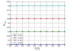
Fig. 9.  $EI_{mm}$  according to different reinforcement ratios ( $\beta_d=0$ ,  $C_t=2.2$ , ACI318)
