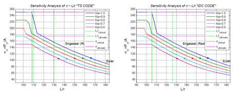
Fig. 15.  $P_u/P_0=1$ ,  $\rho=\%2$ , e=0,  $I_m=0.65I_g$ , left TS code, right IDC code.  $K_w=0.6$  to 1
