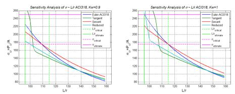
Fig. 12. Buckling stress versus slenderness for various types of modulus theories and ACI-318 code.  $I=1.0 I_g$ , left:  $K_w=0.9$ , right  $K_w=1.0$
