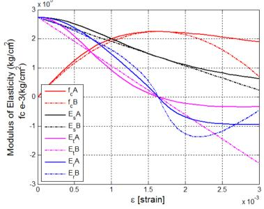
Fig. 2. A: Todeschini model, B: Hognestad model, s: secant modulus, t: tangent modulus, r: reduced modulus of elasticity
