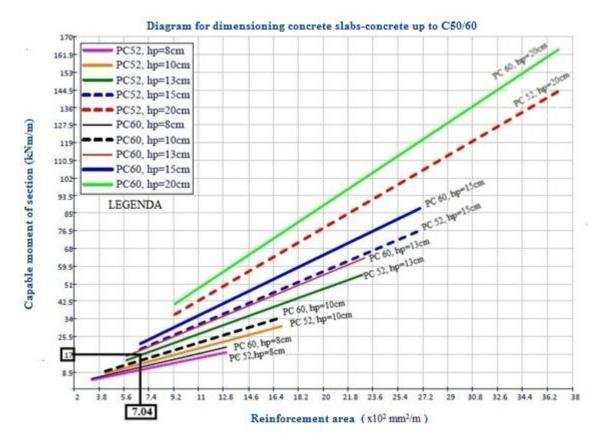
Fig. 3 : Nonomographical diagram for dimensioning concrete slabs - heavy or light reinforced concrete up to C50/60, in accordance with SR EN 1992-1
