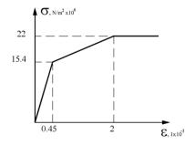
Figure 7. Elastic-plastic model of concrete [6]
