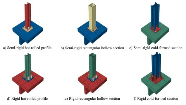
Figure 6: Semi-rigid and rigid base connections
