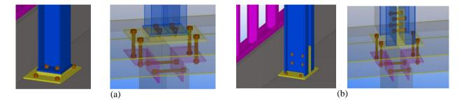
Figure 5. Column-base connection details case 1 and case 3 respectively
