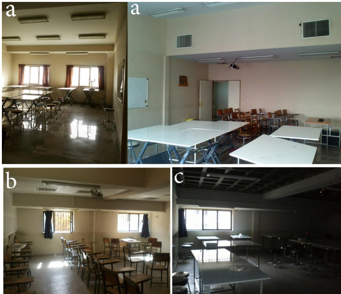
Figure 5: Lighting conditions of south-facing classrooms and ateliers (photos by teh authors) (a) Related to good lighting in ateliers on the third floor, (b) Related to good lighting in one of the classrooms on the first floor and (c) Related to unfavorable lighting in one of the ateliers on the first floor with dark color in ceiling and improper window size and location.
