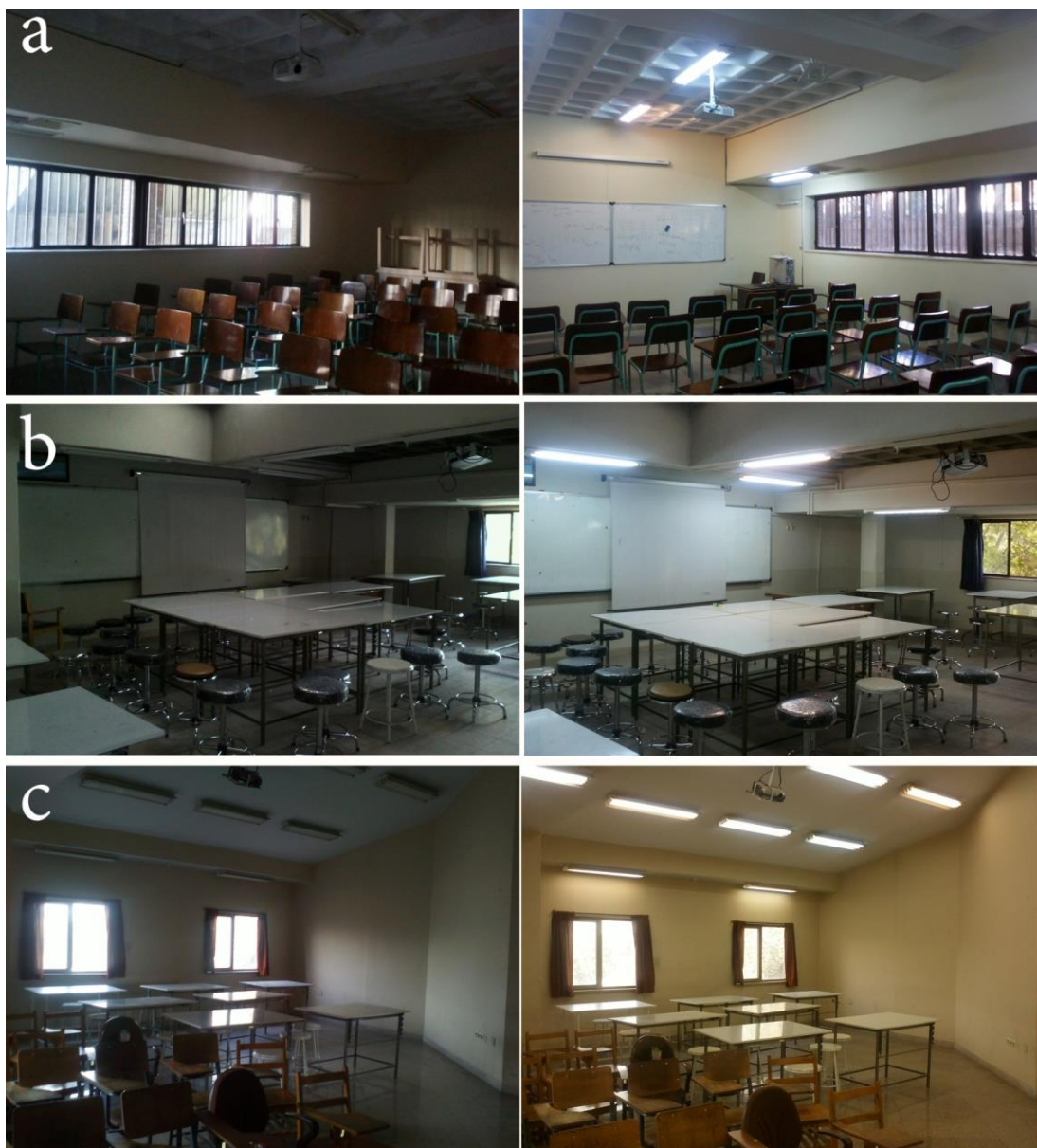
Figure 4: Unfavorable conditions of natural lighting in north-facing classrooms and ateliers and space lighting in the mode of artificial light (photos by the authors) (a) Related to one of the classrooms in the basement, (b) Related to one of the ateliers on the first floor and (c) Related to one of the ateliers on the third floor.
