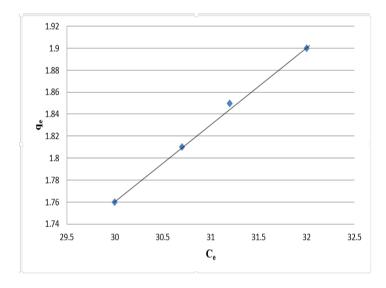
Figure 13. Langmuir Isotherm for Cr Adsorption
