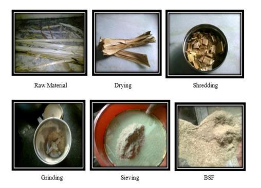
Figure 1. Biosorbent Preparation
