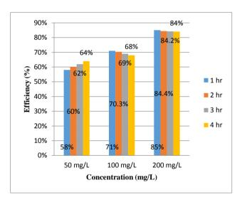
Figure 5. Effect of Concentration on Cr Adsorption
