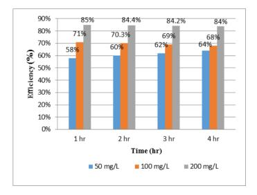
Figure 8. Effect of Contact Time on Cr Adsorption
