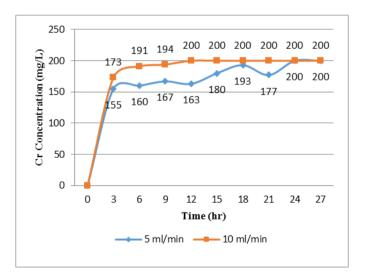
Figure 12. Breakthrough Curves of 10 cm Bed Height on Cr Adsorption
