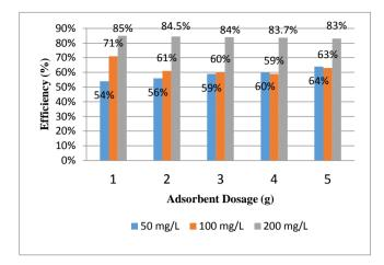
Figure 7. Effect of Adsorbent Dosage on Cr Adsorption
