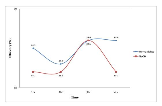
Figure 9. Effect of Modified BSF on Cr Adsorption
