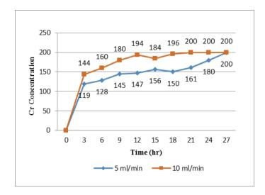
Figure 11. Breakthrough Curves of 20 cm Bed Height on Cr Adsorption
