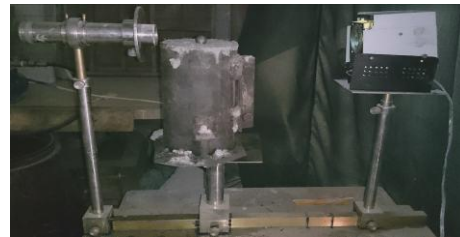
Figure [2] apparatus for measuring plastic Shrinkage
