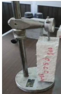
Figure [3] apparatus for measuring dry shrinkage
