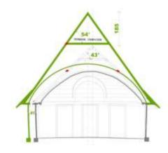
Figure 5. Simulation of the original shingle section.
