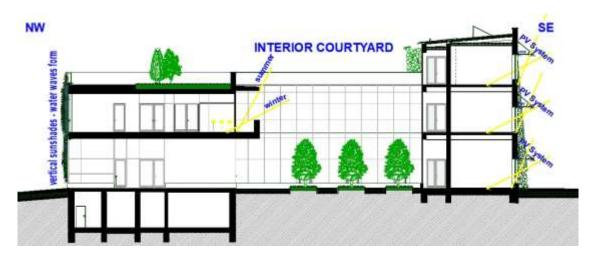
Figure 4. Section with metal structures designed for actual horizontal sunshades and a potential future photovoltaic system on the South-East elevation and vertical sunshades on water waves form on North West elevation (2)
