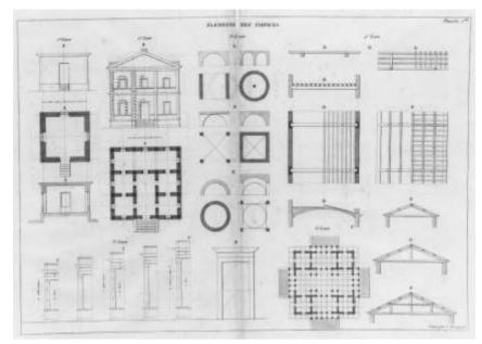
Figure 1. The logical decomposition of buildings into formal elements. (J. N. L. Durand, Précis des leçons d'architecture données à l'École Royale Polytechnique. Paris: J.N.L. Durand, 1802.)
