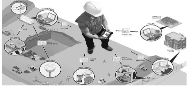
Figure 2: Combination of Positioning Systems and Information Technology in Construction Source: [25]
