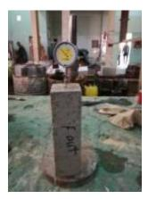
Figure (3) Apparatus for measuring drying shrinkage.
