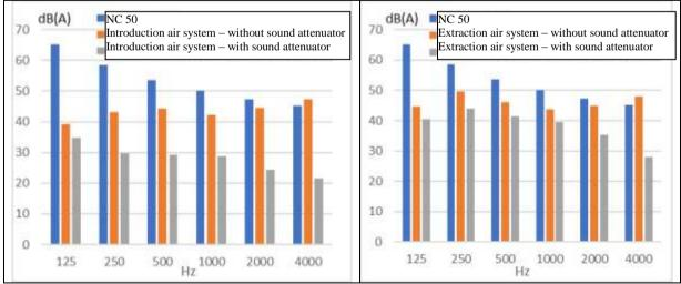
Figure 7. Sound pressure levels [dB] for inlet air diffusion and extraction air
