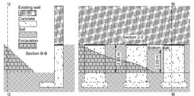
Figure 7. Mechanical shovel excavation
