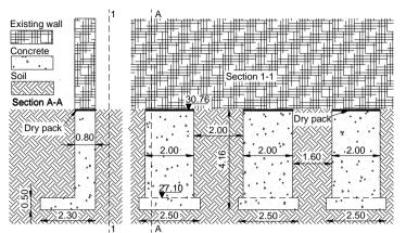
Figure 4. Underpinned pits pouring
