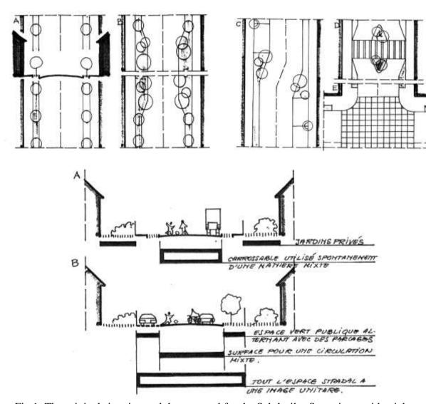
Fig.1: The original situation and the proposal for the Salcâmilor Street in a residential area of Timişoara (original drawings)
