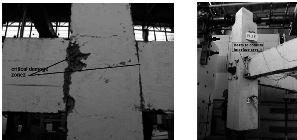
Figure 1 Hybrid joints; critical interface zones: (1) Planar model; (2) Spatial model
