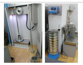
Proctor apparatus (Froewag) and sieve shakers (Matest S.p.A) in order to determine the degree of compaction and grain size distribution for transportation infrastructures.
