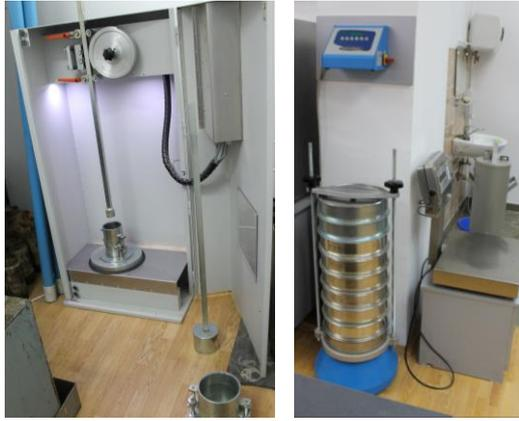
Proctor apparatus (Froewag) and sieve shakers (Matest S.p.A) in order to determine the degree of compaction and grain size distribution for transportation infrastructures.
