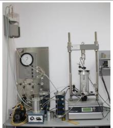
Complete Triaxial System (Controls) – The most advanced technology for soil properties determinations such as: permeability, soil strength, consolidation. It provides software in order to analyze and determine soil parameters.
