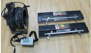
Portable horizontal and vertical inclinometers (Durham Geo-Enterprises) used to monitor subsurface movements and deformations.
