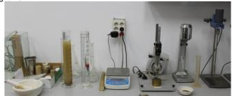
Small apparatus used to determine soil physical properties in order to classify soil types.
