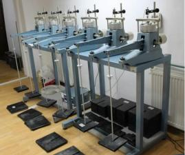
Oedometers, front loading (Controls) - determines the rate and magnitude of consolidation of a soil specimen restrained laterally and subjected to a number of successive increments of vertical loads, provided with Data acquisition system (Controls) and software programs.
