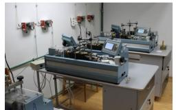
Five automatic shear testing machines (Controls), ideal for research purposes, in order to determine the soil mechanical parameters for consolidated, unconsolidated, drain and undrain conditions
