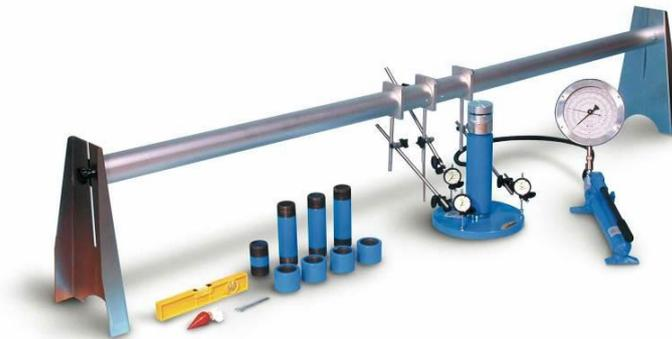
Static plate bearing test equipment (Matest) used for the determination of the bearing capacity of a soil in-situ on road constructions, foundations, road subgrades, airport and highway pavements.
