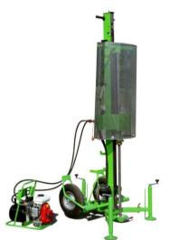
Dynamic Probing Rig-DPSH (Geotool) for in-situ testing, in order to determine soil mechanical parameters at different depths.
