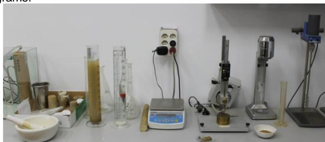
Small apparatus used to determine soil physical properties in order to classify soil types.
