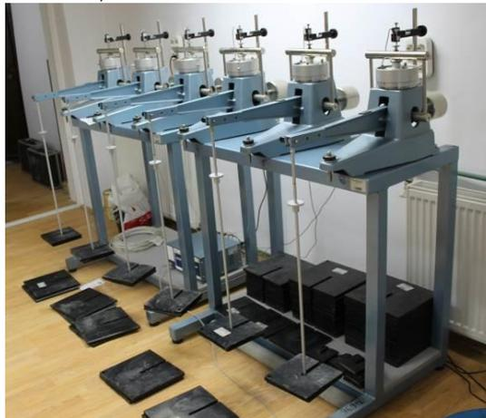
Oedometers, front loading (Controls) - determines the rate and magnitude of consolidation of a soil specimen restrained laterally and subjected to a number of successive increments of vertical loads, provided with Data acquisition system (Controls) and software programs.
