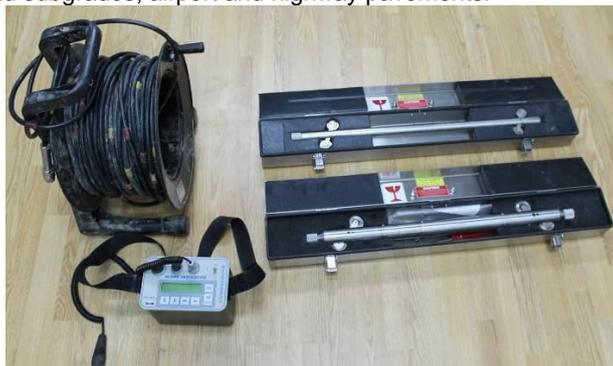
Portable horizontal and vertical inclinometers (Durham Geo-Enterprises) used to monitor subsurface movements and deformations.
