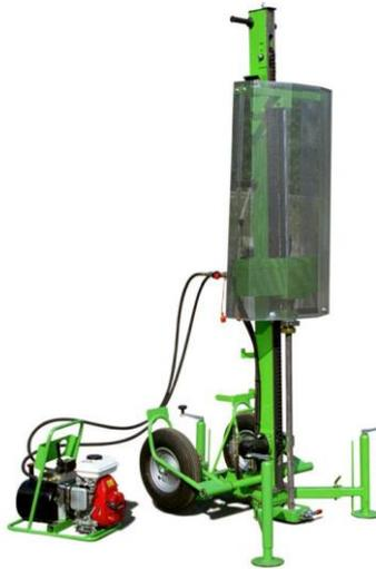
Dynamic Probing Rig-DPSH (Geotool) for in-situ testing, in order to determine soil mechanical parameters at different depths.
