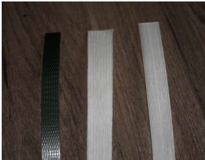
Fig. 4.1- Benzi sintetice tip cordstrap a)PET b) fibre de poliester c) fibre de poliester laminate
