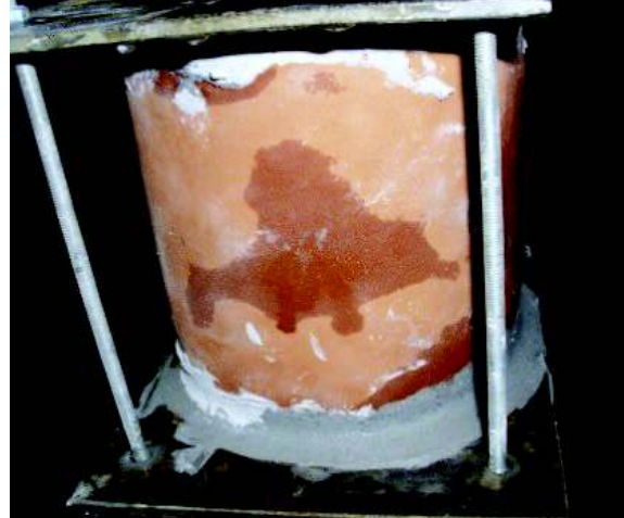
b. pipe P4 water leakage at 3.5 bar
