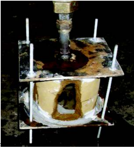
c pipe P3 under pressure of 1.0bar
