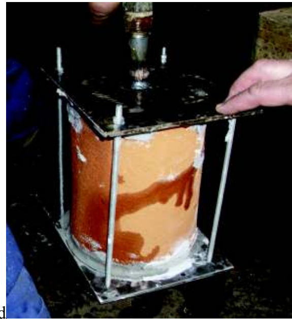
d. pipe P4 under under 1.2 bar
