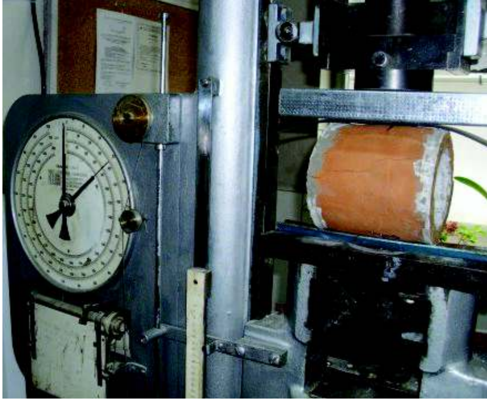
Figure 4.16: Crushing test set up
