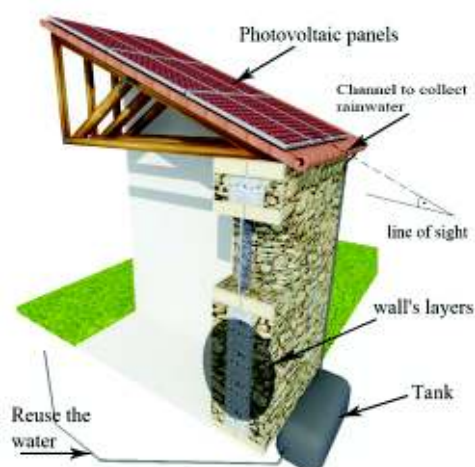
Figure 4.24: Energy efficiency by implementing solar energy and re-use of water
