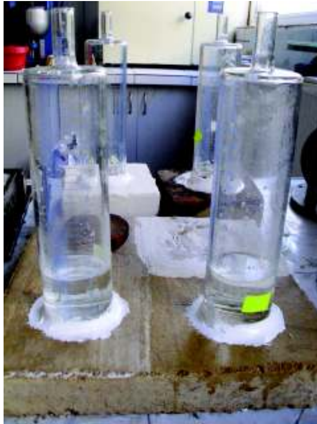
Figure 4.11: Waterproof testing of treatment materials
